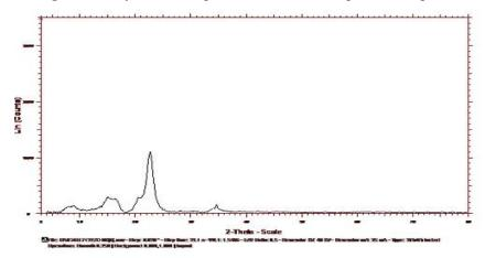
Figure 8: X-Ray Diffraction pattern of Ezetimibe LSC formulation without drug
